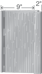
11" BOARD & BATTEN SIDING
